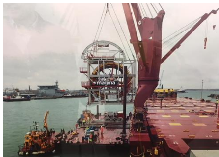
IDP deployment: auxiliary drill pipe
